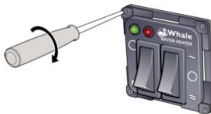
Fig. 18 Secure Control Panel
