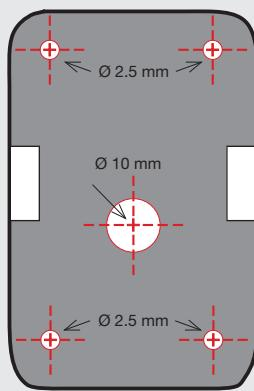
Find a suitable spot for the camera on the back of your motorhome. The optimum height is about 2.5 m from the ground.
