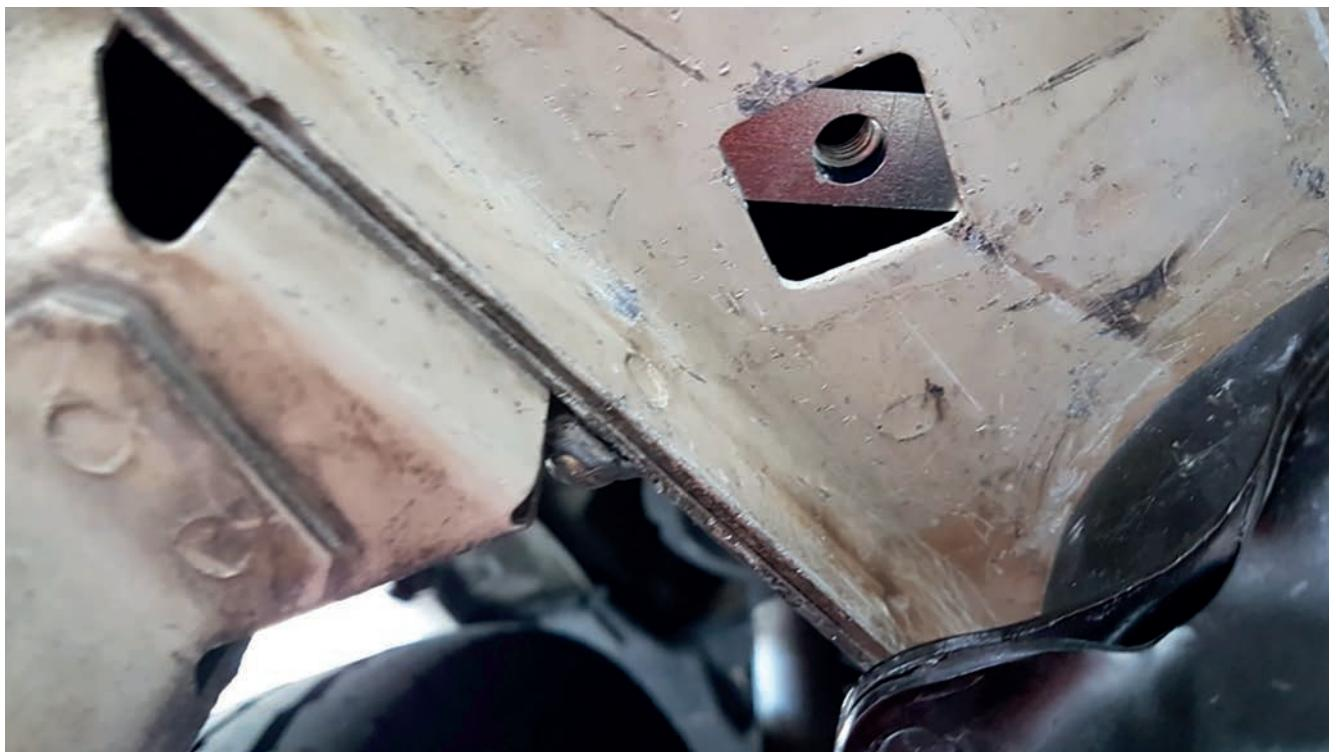
Insert the mounting plate with the screw hole concentric to the square hole in the chassis.
